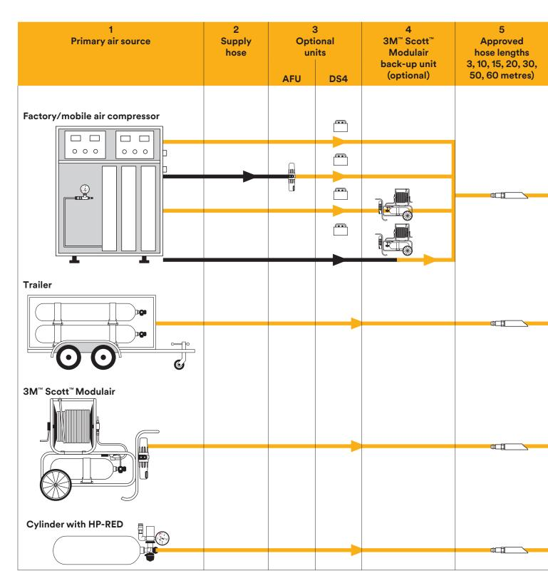
These examples are designed to give an indication of how an airline system can be built up. Please note that many other configurations can be specified. The line drawings above are only representations of 3M™ Scott™ airline equipment and should not be considered exact specification. Maximum length of hose to the user after the 3M™ Scott™ Modulair should be no more than 105 metres. Please see Modulair user manual for approved configurations.
