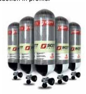
The engineers of 3M™ Scott™ determined the best manner to accomplish this was to increase the pressure of the cylinders to 379 bar, which created the new 379 bar cylinders, an "industry first." The result is a cylinder that has more than a 10% reduction in weight and profile in a traditional form familiar to BA users.
